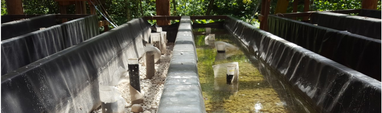
Figure 1: The “Hyporheos:::Rinnen” for the investigation of the stream bottom during an experiment about drying: on the left dry and on the right with water flowing through.
