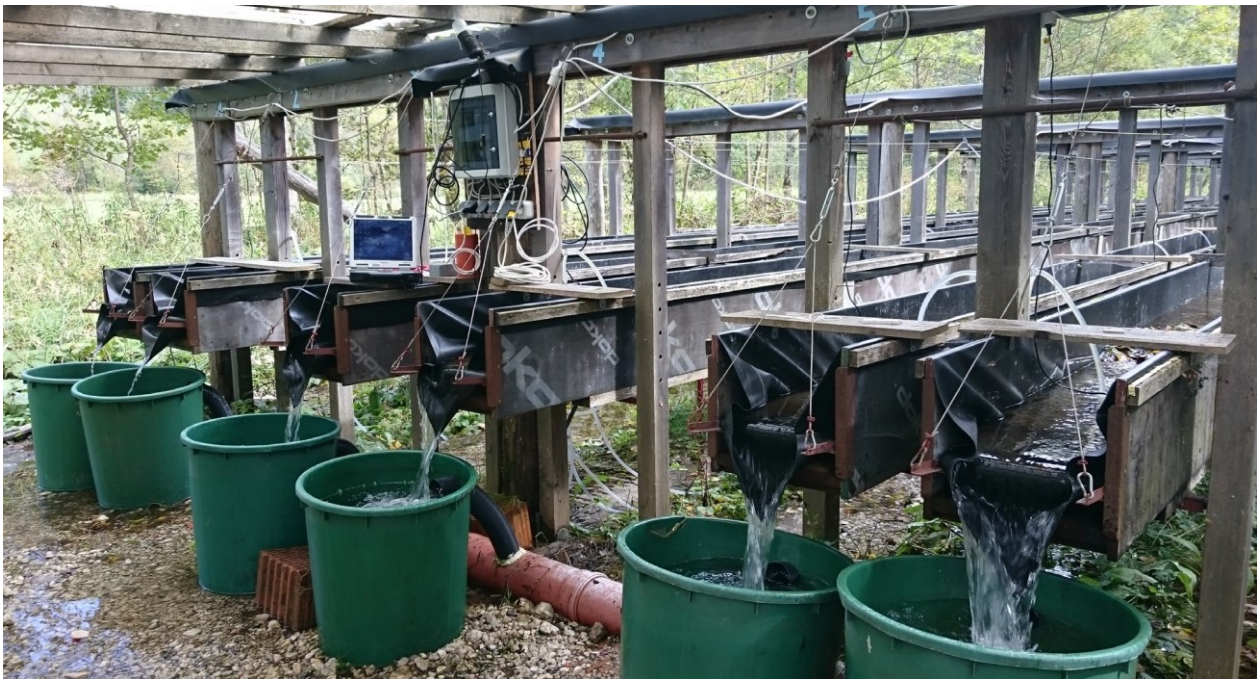
Figure 2: The “Lunzer:::Rinnen” during an experiment with different water flow velocities. (increasing water flow from left to right)
